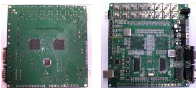
Figure 3. Board II: IEC 62.132-4 std compliant board comprised of 6 layers for conducted immunity measurement. Views: (a) Top; (b) Bottom.
