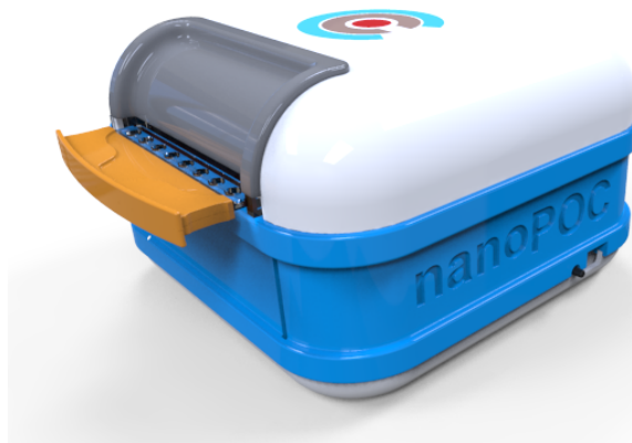
Fig. 3: Device prototype printed in ABS.
