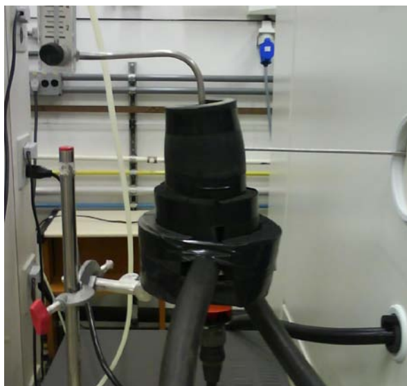
Figure 2 – Transfer Standard Sensor Connected at INMETRO Climatic Chamber and Cooled at -3\text{ }^{\circ}\text{C}
