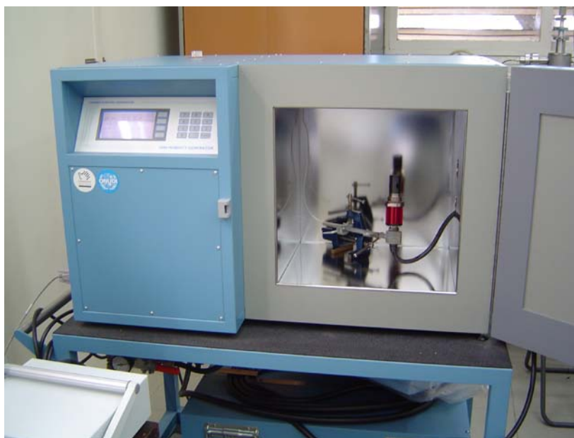
Figure 3 – Transfer Standard Sensor Inside of the Chamber of INTI Primary Generator
