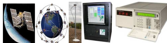
Fig. 1. From left to right: GPS satellite, GPS constellation, SIM antenna and time transfer system, caesium clock.
