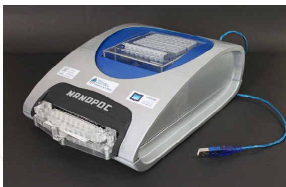
Fig. 12. Point of care electrochemical immunosensing platform Nanopoc®, designed for the diagnosis of foot-and-mouth disease, brucellosis, and Chagas disease (Longinotti et al., 2011). The sample preparation is carried out in the blue sector, which involves magnetic separations. The final amperometric measurement is carried out in the 8-channel electrochemical cells at the front of the device. Data are processed by a PC via a USB connection.
