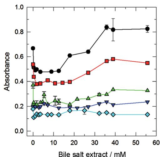
Fig. 8 Effect of the BSE concentration on the absorbance of HSPC/CHOL liposomes (black circle: 1.04 mM; square: 0.76 mM; up triangle: 0.5 mM; down triangle: 0.36 mM; diamond: 0.25 mM) after 1 hour of incubation at 37 °C.
