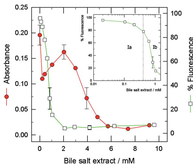
Fig. 1 Absorbance (circles) and fluorescence (squares) changes of suspensions of SPC liposomes (0.60 mM) in the presence of BSE after 1 h of incubation at 37 °C. The inset corresponds to low concentrations of BSE.
