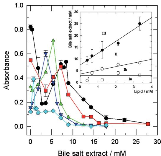
Fig. 6 Solubilisation curves of HSPC liposomes (circle: 3.33 mM; square: 2.13 mM; up triangle: 1.24 mM; down triangle: 0.67 mM; diamond: 0.40 mM) obtained in the presence of BSE after 1 h at 55 °C. Inset: the phase diagram of HSPC/BSE mixtures obtained from the solubilisation curves. (\*: Point rejected).
