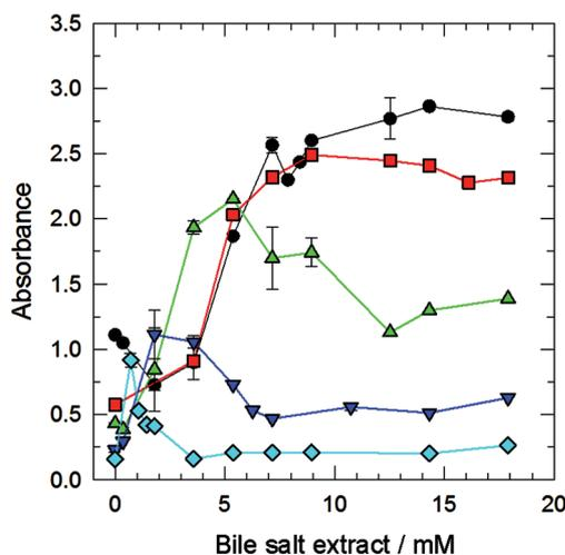
Fig. 5 Effect of the BSE concentration after 1 hour of incubation at 37 °C on the absorbance of HSPC liposomes (circle: 3.33 mM; red square: 2.13 mM; up triangle: 1.24 mM; down triangle: 0.67 mM; diamond: 0.40 mM).
