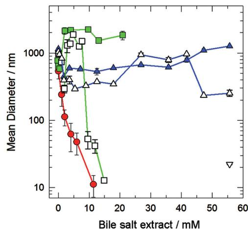
Fig. 3 Effect of the BSE concentration on the mean diameter (%volume distribution) after 1 hour of incubation of SPC (circle: 1.8 mM, 37 °C), HSPC (dark square: 1.2 mM, 37 °C; white square: 3.3 mM, 55 °C), and HSPC/CHOL liposomes (dark up triangle: 1.1 mM, 37 °C; white up triangle: 1 mM, 65 °C). The mean diameter of HSPC/CHOL liposomes incubated with 56 mM BSE at 65 °C is also expressed as number distribution (white down triangle).
