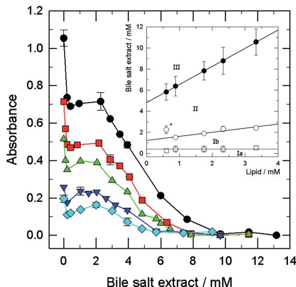
Fig. 2 Solubilisation curves of SPC liposomes (circle: 3.33 mM; square: 2.33 mM; up triangle: 1.75 mM; down triangle: 0.88 mM; diamond: 0.60 mM) obtained in the presence of BSE after 20 min at 37 °C. Inset: the phase diagram of SPC/BSE mixtures obtained from the solubilisation curves. (\*: Point rejected).
