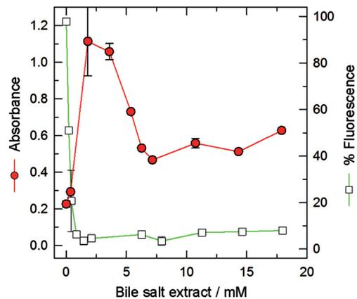
Fig. 4 Absorbance (circle) and fluorescence (square) changes of suspensions of HSPC liposomes (0.67 mM) in the presence of BSE after 1 h of incubation at 37 °C.
