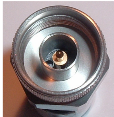
Figura 10b: Conductor externo sin ranuras (slotless)
