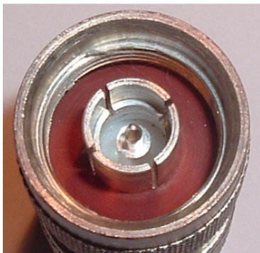
Figura 10a: Conductor externo ranurado (slotted)
