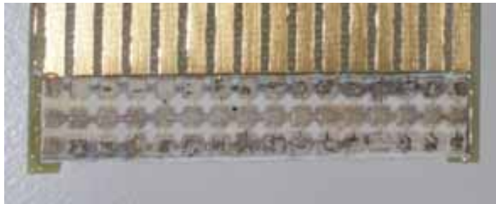
Mounting of a linear array for testing
