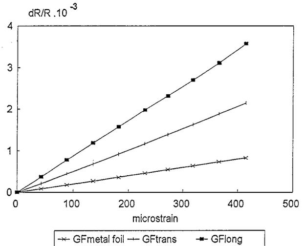
Fig. 2. Relative change of resistance as a function of longitudinal and transversal strains.
