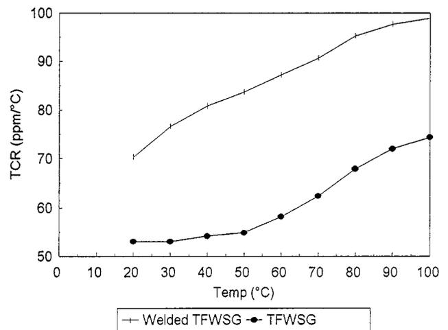
Fig. 3. TCR as a function of temperature for a TFWSG with stainless-steel carrier.
