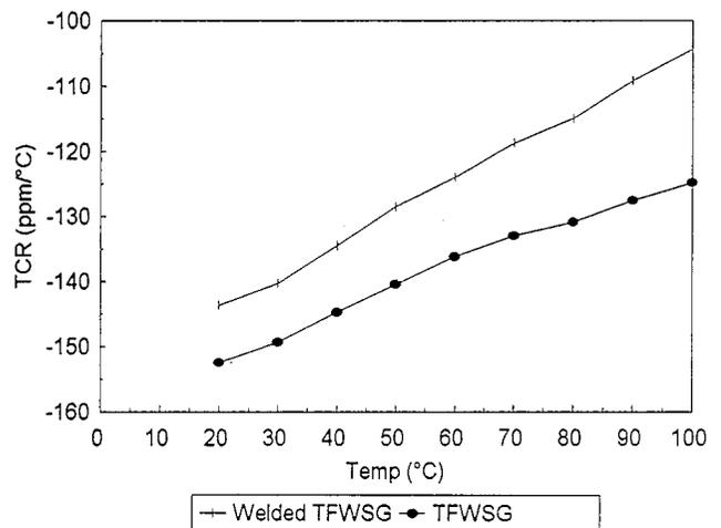
Fig. 4. TCR as a function of temperature for a TFWSG with titanium carrier.
