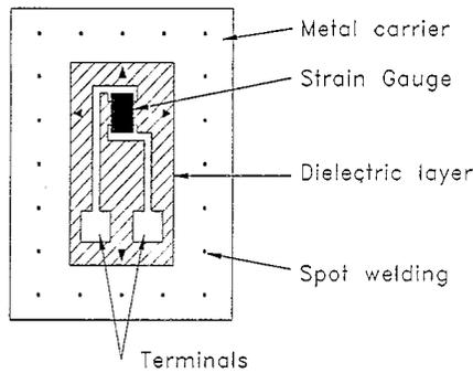
Fig. 1. Layout of a TFWSG. The size of the thick-film resistor is 1.6 mm × 1.6 mm.
