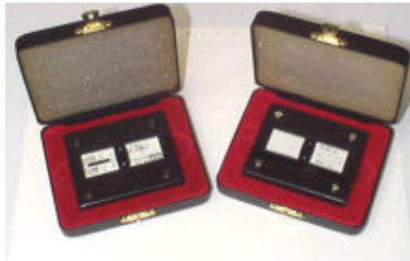
Figure 3: NRC step height and roughness specimens in their cases
