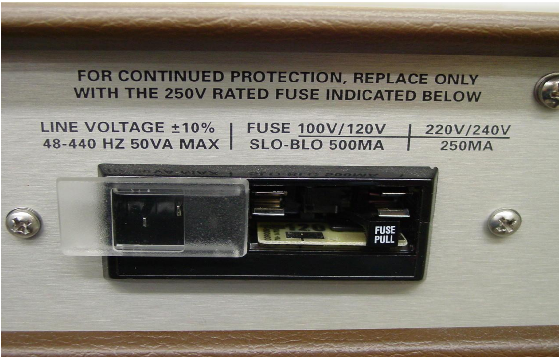
Figure I2. Rear view of AH1100 Enclosure with fuse removed
