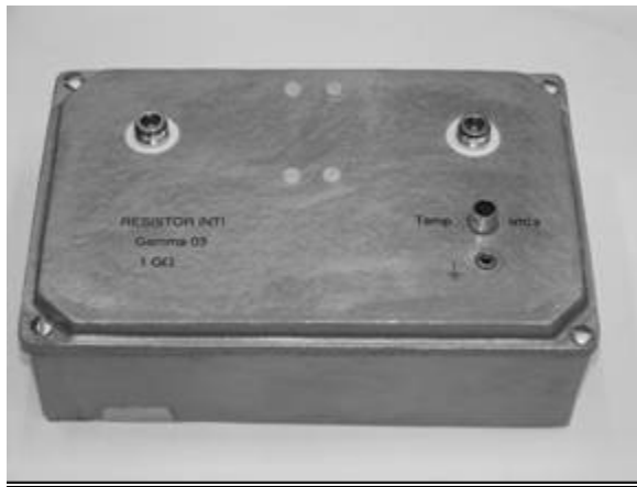
Figure 2. 1 GΩ INTI's resistors
