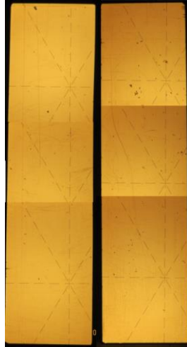
Figure 7. Aspect of the measuring faces of the 100 mm Steel GB at the end of circulation.
