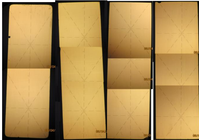
Figures 8, 9, 10 and 11. Aspect of the measuring faces of the 10, 50, 75 and 100 mm Ceramic GB at the end of circulation.
