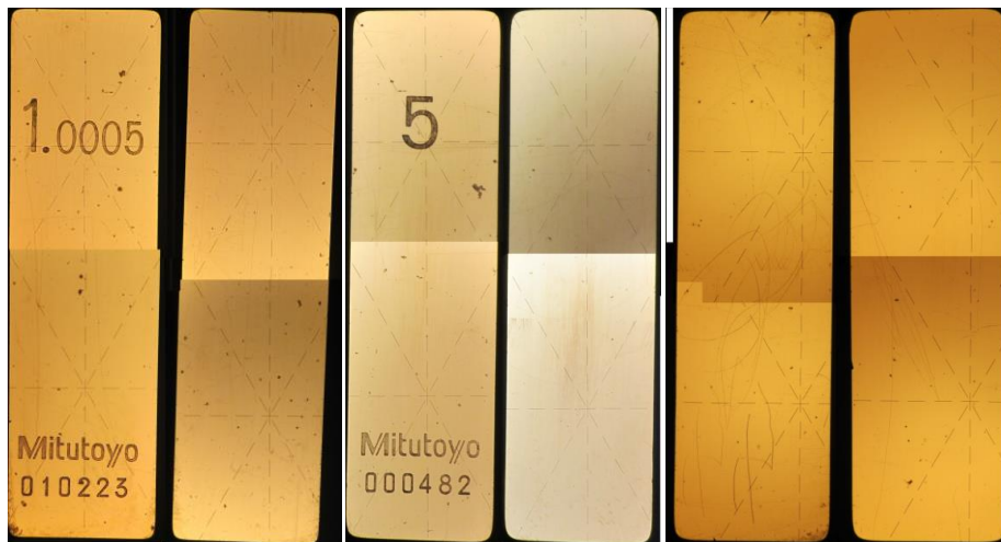
Figures 1, 2 and 3. Aspect of the measuring faces of the 1.000 5, 5 and 7 mm Steel GB at the end of circulation.
