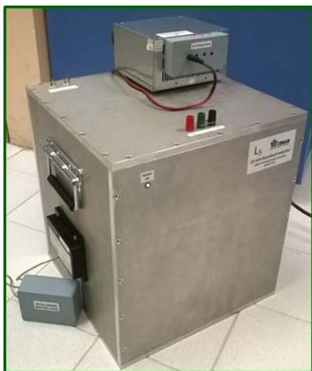
Figure 1 Temperature controlled enclosure used in the SIM.EM-K3 comparison.
