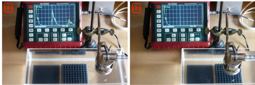
Figure 4. Reflection loss measurement setup. The acoustic pressure reflected as compared to that reflected from a 304-stainless-steel reference block. Left (a): The reference block has reflectivity of 0 dB down. The reference is the signal reflected from the surface of the reference block with the same area as the sample (not shown in the photo). The bottom plate has a reflectivity of -7 dB; Right (b): The sample of PSA reflects one fortieth of the energy which reflects the bottom plate.
