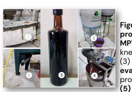
Figure 7: OBC production process MPV 2. (1) thermokneader (2) decanter (3) sedimentation (4) evaporation, equipment provided by INTI (5) fractionated OBC.
