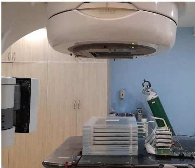
Figure 11 - LINAC and the acquisition system setup.
