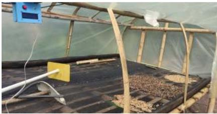
Fig. 10: Installation of the electronic system in the dryer.
