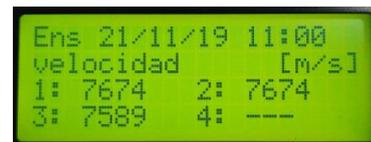
Fig. 6. Values on the VOD meter display.
