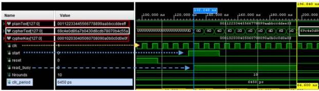
Fig. 3. AES-128 Vivado simulation with FIPS197 test vectors.
