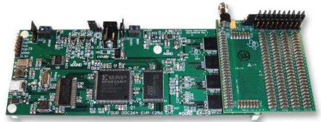
Figure 4 - DDC264EVM Main data acquisition board.
