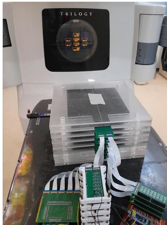
Figure 6 - Connectivity of the acquisition system.
