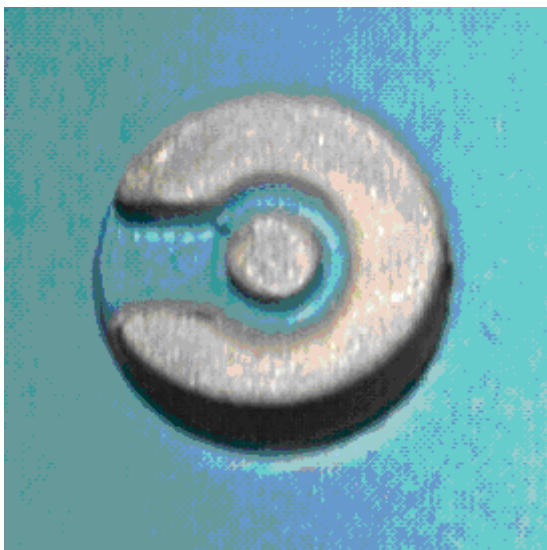
Figure 2. Thick film electrode in a LTCC cell.
