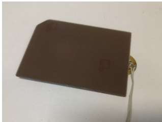
Fig. 1. Impact plate sensor. A piezoelectric sensor is glued to the fiberglass plate.
