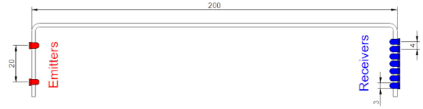
Fig. 2. Infrared sensor frame. Two infrared emitters on the left (red) and seven infrared receivers on the right (blue).
