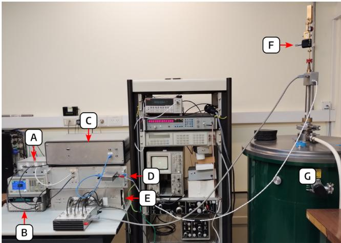
Fig. 2. INTI's AC-QVM. A: Clock generator. B: Signal generators. C: DUT. D:  $\Sigma\Delta$  digitizer. E: Programmable current source. F: Microwave generator. G: Liquid Helium dewar where the Josephson array is cooled down to 4.2 K. A and F are locked to INTI's Cesium atomic clock frequency.
